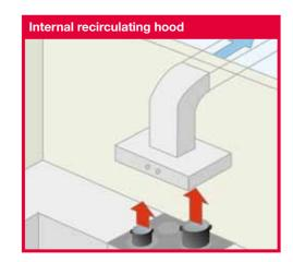
**Recommended filters:** - anti-odour activated carbon filter - cut-to-fit anti-grease filter
